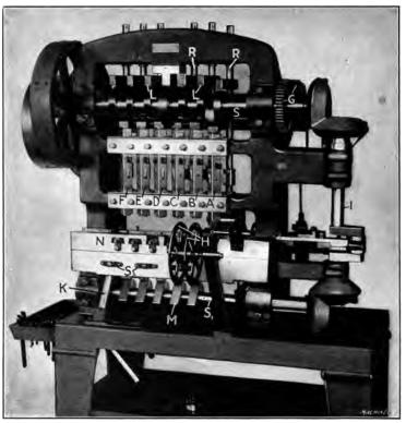
Fig. 1. Multiple Plunger Press
